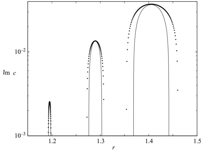
FIGURE 4. Imaginary part of the phase speed  $\text{Im } c$  as a function of  $r$  (in linear–logarithmic scale) for the KW–KW instability in anticyclonic flows with  $s = 0.1$ . Numerical (dots) and asymptotic (solid curves) results are compared for  $\epsilon = 0.3, 0.4, 0.5$  (with increasing  $\text{Im } c$ ), and  $\theta = \pi/2$  (i.e.  $k = 0$  and  $m = r$ ).
