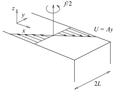
FIGURE 1. Schematic of the Couette flow, with velocity  $(Ay, 0, 0)$ , of a three-dimensional Boussinesq fluid with constant Brunt–Väisälä frequency  $N$ . The domain rotates around the (vertical)  $z$ -axis at rate  $f/2$ ; it is unbounded in the  $x$ - and  $z$ -directions, and bounded in the  $y$ -direction by two rigid walls separated by a distance  $2L$ .
