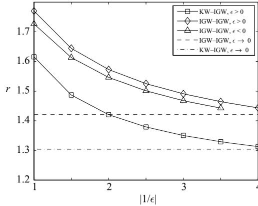
FIGURE 7. Numerical estimates of the value of  $r = (k^2 + m^2)^{1/2}$  which maximizes  $\text{Im } c$  for KW–IGW and IGW–IGW instabilities as a function of  $1/|\epsilon|$  for  $s = 0.1$ . The asymptotic limit for  $\epsilon \rightarrow 0$  obtained from (4.11) and (4.13) are also shown.
