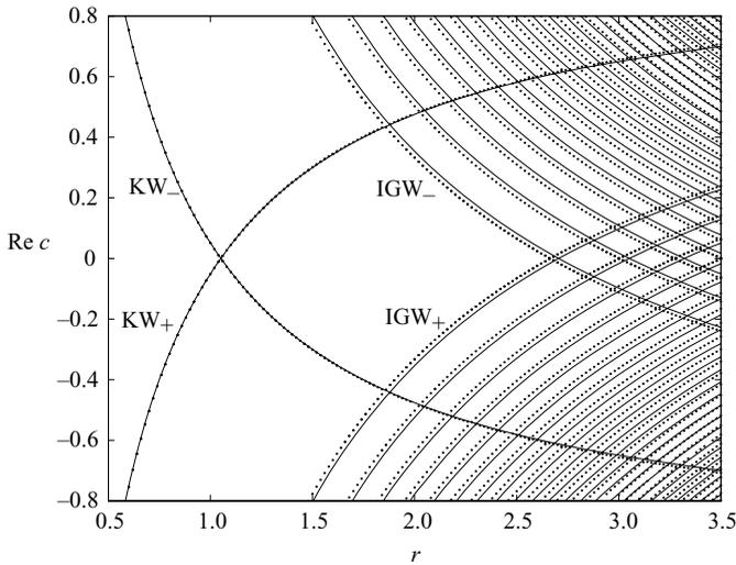
FIGURE 2. Dispersion relation for an anticyclonic flow, with  $\epsilon = 0.1$ ,  $\delta = 2$  and  $s = 0.1$ . The two Kelvin waves (KW) are shown along with many inertia-gravity waves (IGW). The asymptotic estimates for  $|\epsilon| \ll 1$  (solid curves) are compared with numerical solutions (dotted curves).
